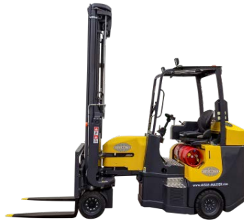
c) Articulated forklift. Source: [18]
