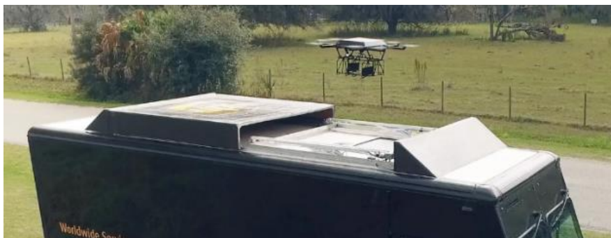
Figure 7. UPS delivery drone that can land on top of a courier car [16]
