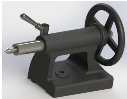
Figure 3. Tailstock with manual body with retractable barrel (Source: https://www.smartlathe.com )
