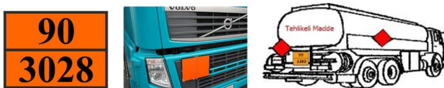
Figure 2. Hazard Signs and their Placement.
