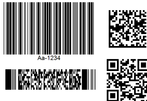
Figure 1. barcode and 2D code examples (Code39, datamatrix, PDF417, QRCode) [9]
