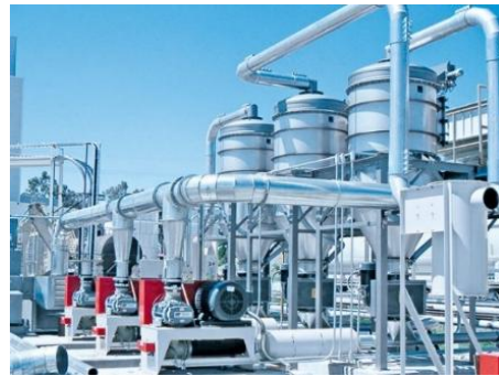
b) Pneumatic conveyor system, source: [8]
