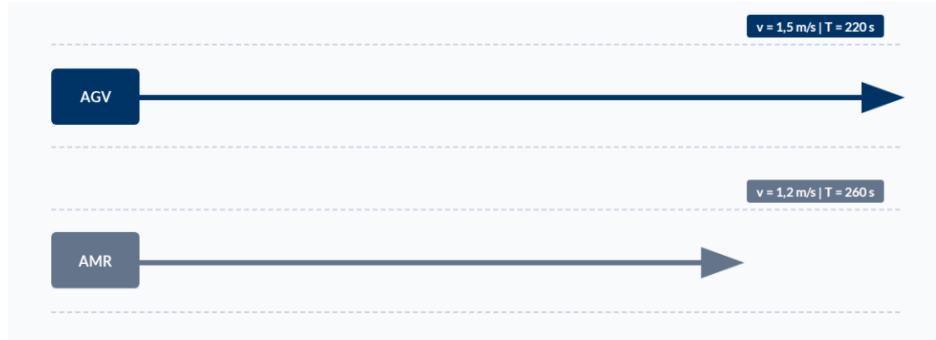
Figure 6. Comparison of AGV and AMR cycle times in an ideal, accessible environment (own edited)
