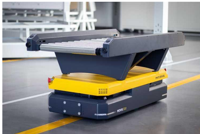
Figure 1. Automated Guided Vehicle (AGV) using line tracing [8]
