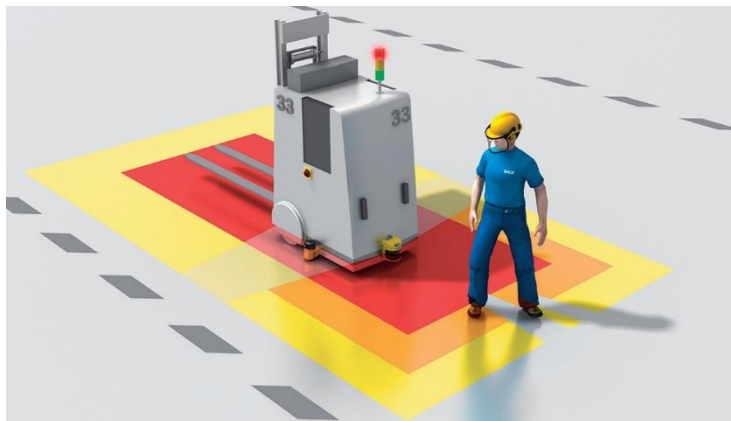
Figure 5. Dynamic safety zones for autonomous vehicles: warning (yellow) and protective field (red) [19]
