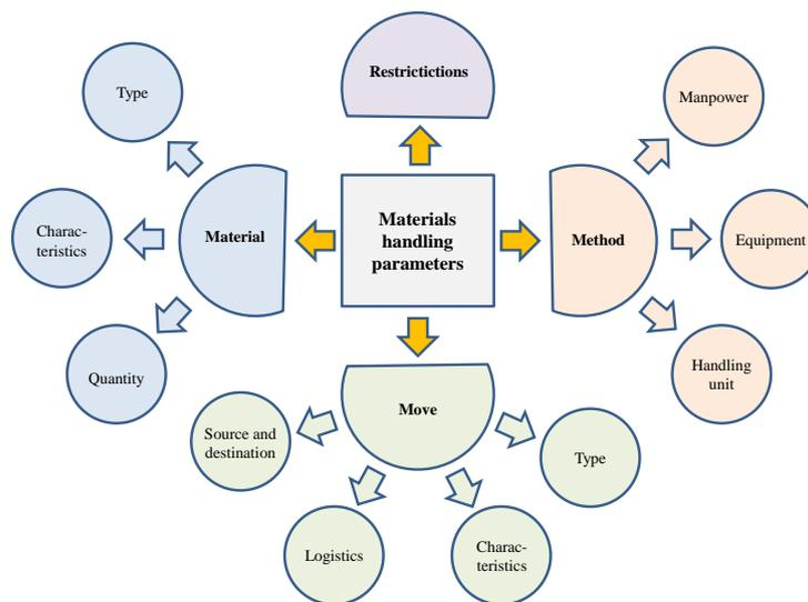
Figure 2. Material handling factors based on [13]
