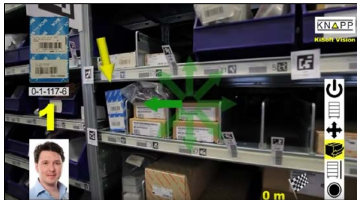
Figure 15. KNAPP KiSoft Pick by Vision system, source: KNAPP
