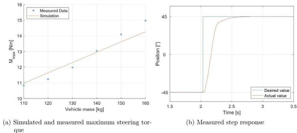
Figure 8. Recorded and simulated steering values
