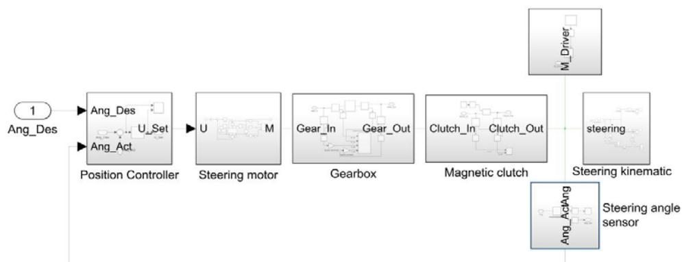
Figure 5. Overall simulation model of the steering system
