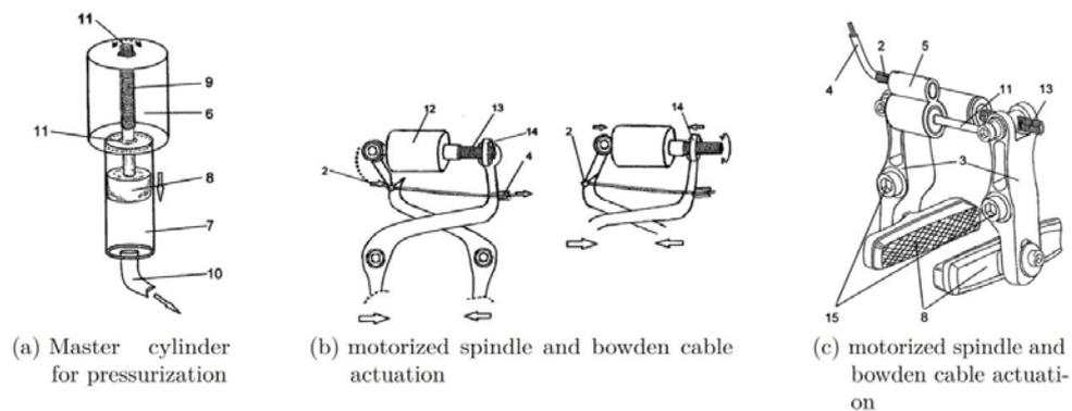
Figure 2. Patented automated brake actuation [8]-[10]
