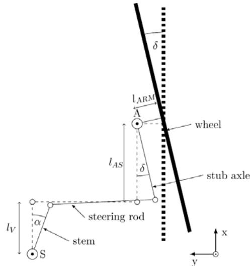
Figure 4. Modelling of the steering mechanics
