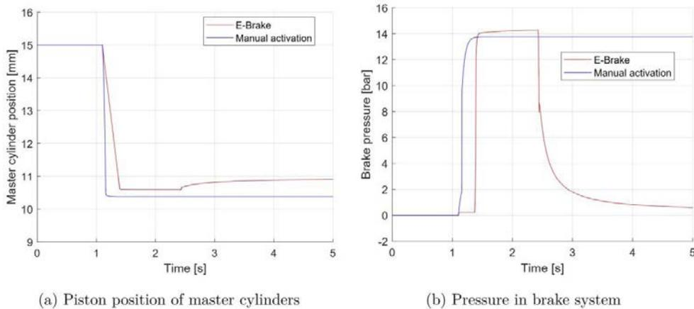
Figure 9. Manual and electromechanical brake activation
