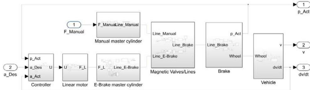
Figure 7. Overall simulation model of the braking system
