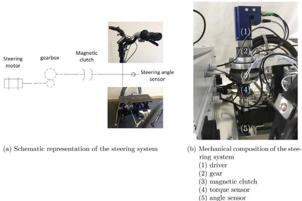
Figure 3. Automated steering of the test vehicle
