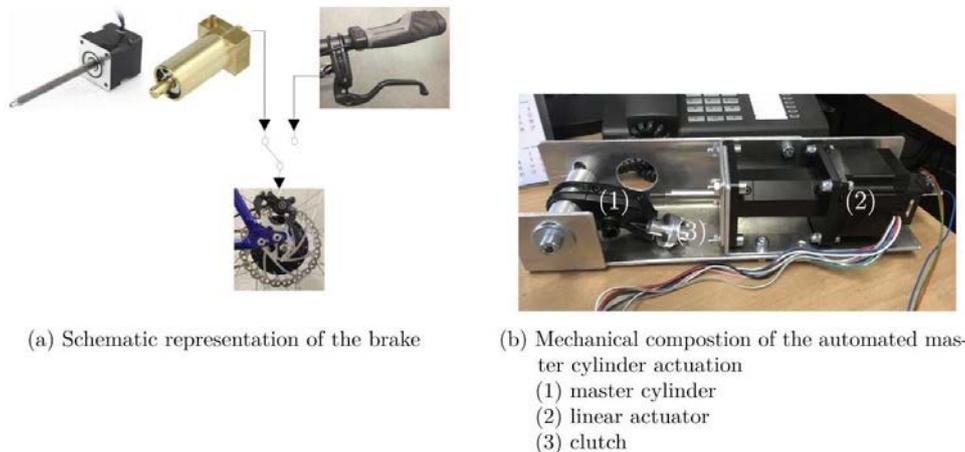
Figure 6. Automated brake of the test vehicle
