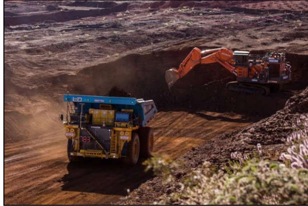
Figure 9. 416 tons Komatsu dumper [26]
