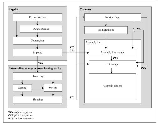
Figure 1. Multilevel cross docking supply
